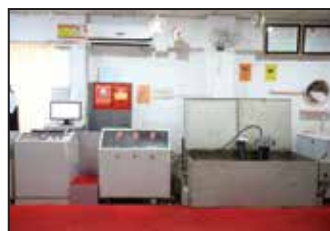
Hydrostatic Pressure Test
