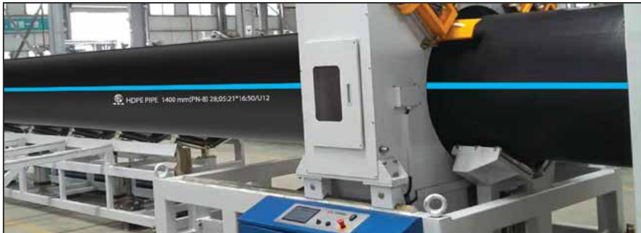
1400 mm RFL HDPE Pipe Production
